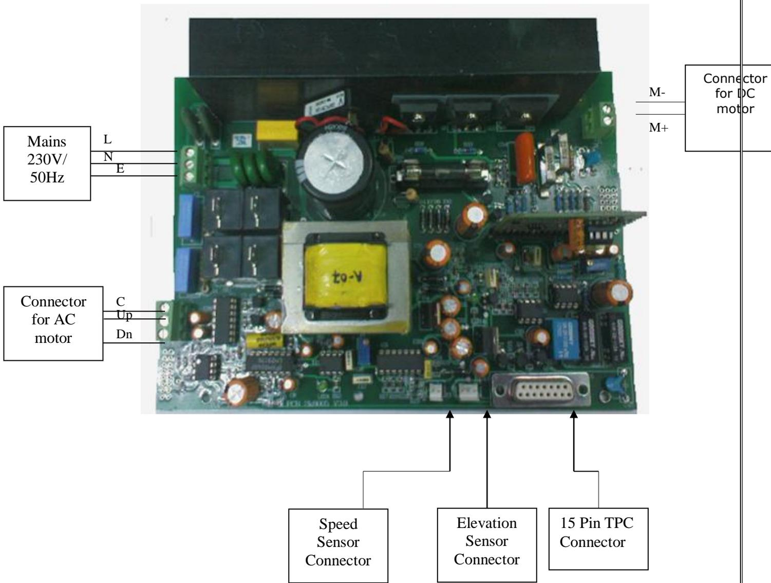
**Fig 7. High frequency drive connections**
