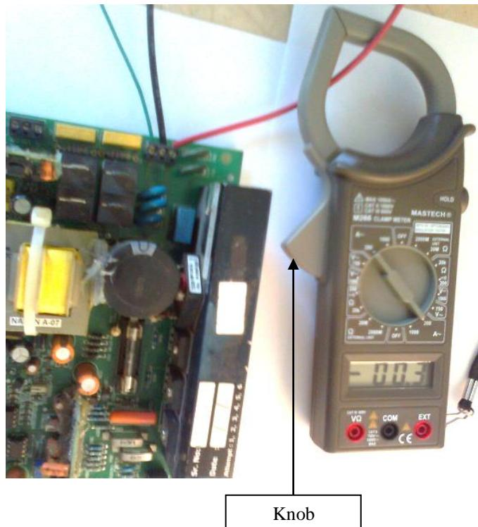
**Fig10. Clamp meter connected with high frequency drive to measure AC current.**
