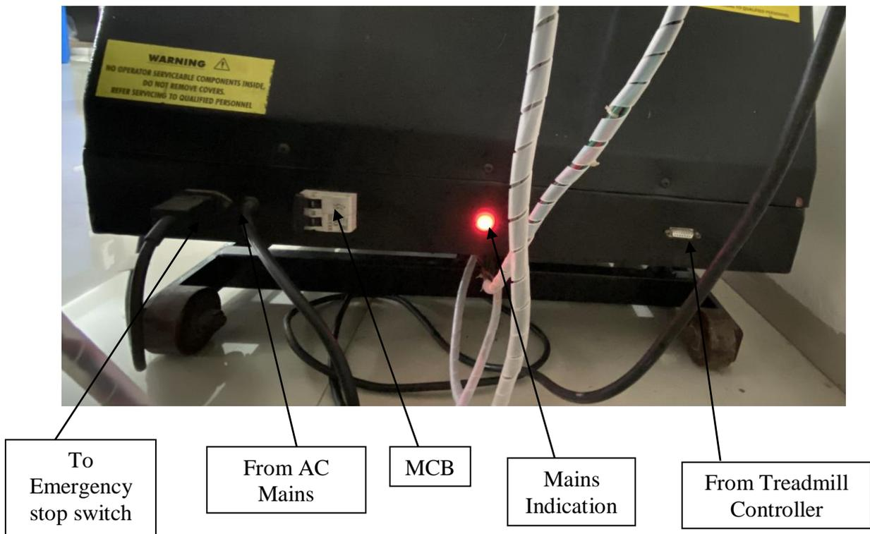
Fig 6. FRONT PANEL CONNECTION
