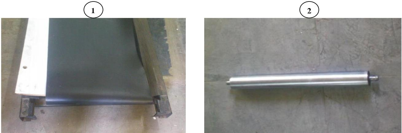
**Fig.15. Treadmill after removing the back roller**
