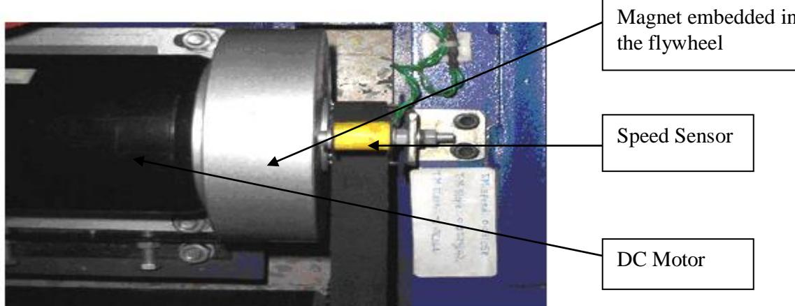
**Fig 4. SPEED SENSOR**
