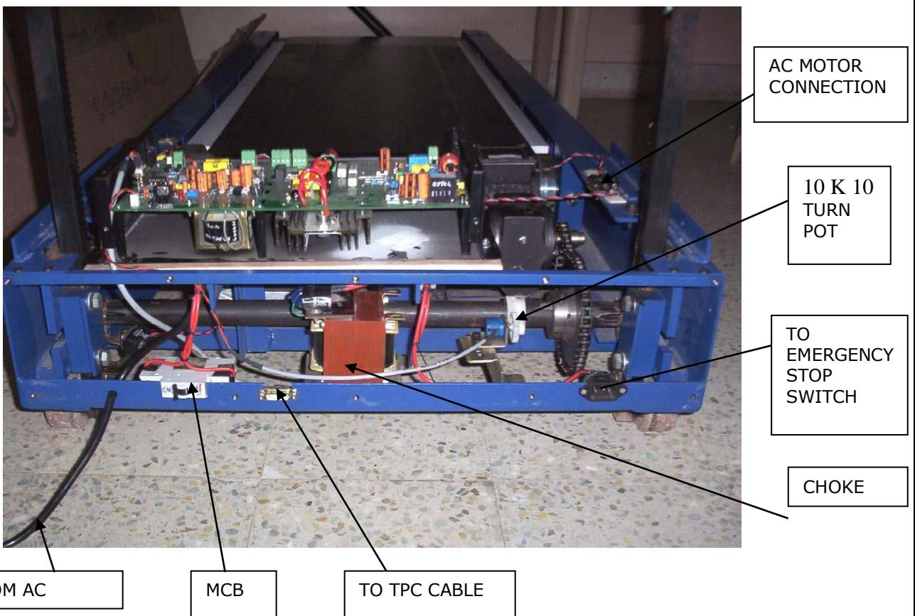
**Fig 6. FRONT PANEL CONNECTION**
