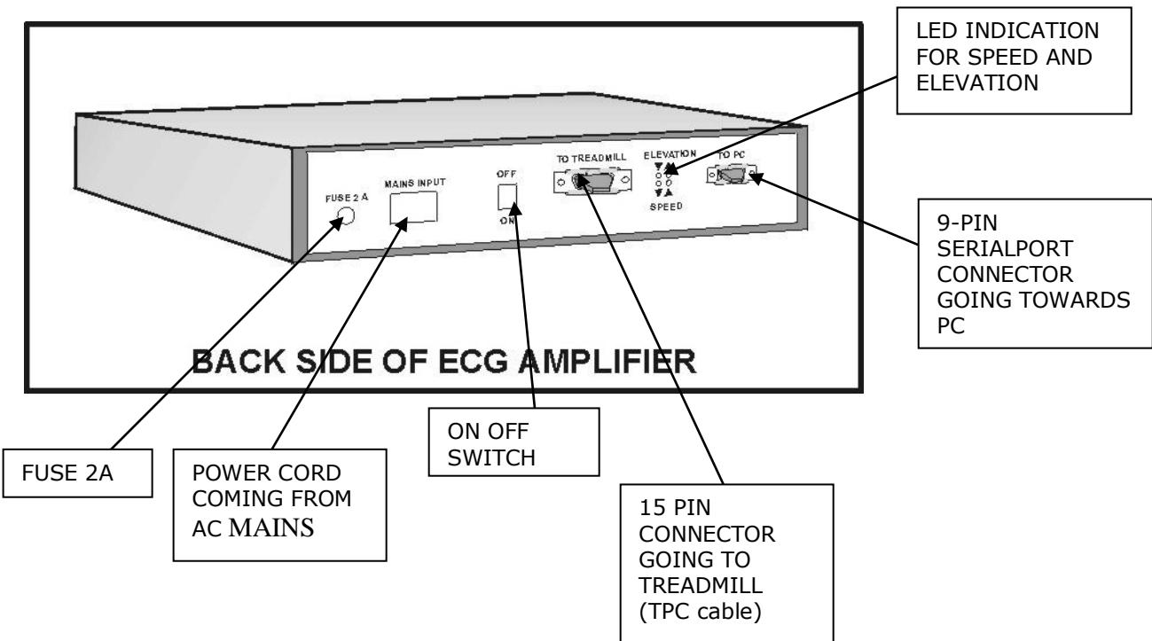
**Fig 2. AMPLIFIER CONNECTIONS**
