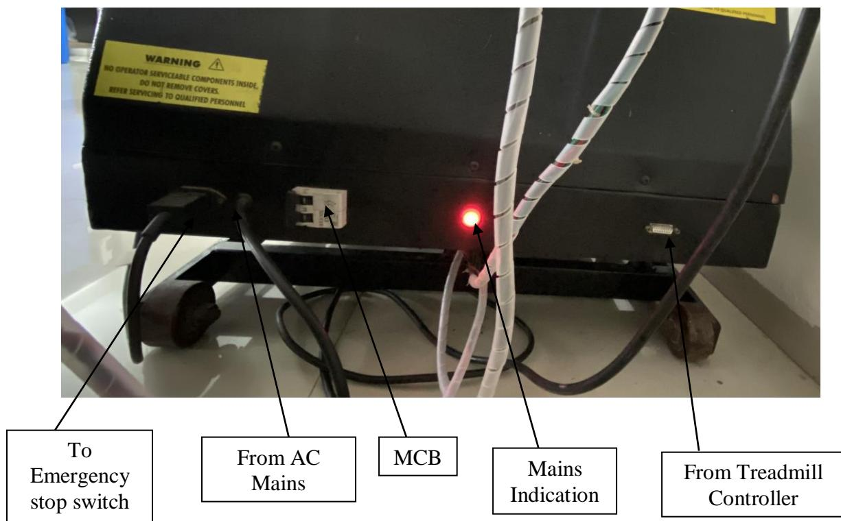
**Fig 6. FRONT PANEL CONNECTION**
