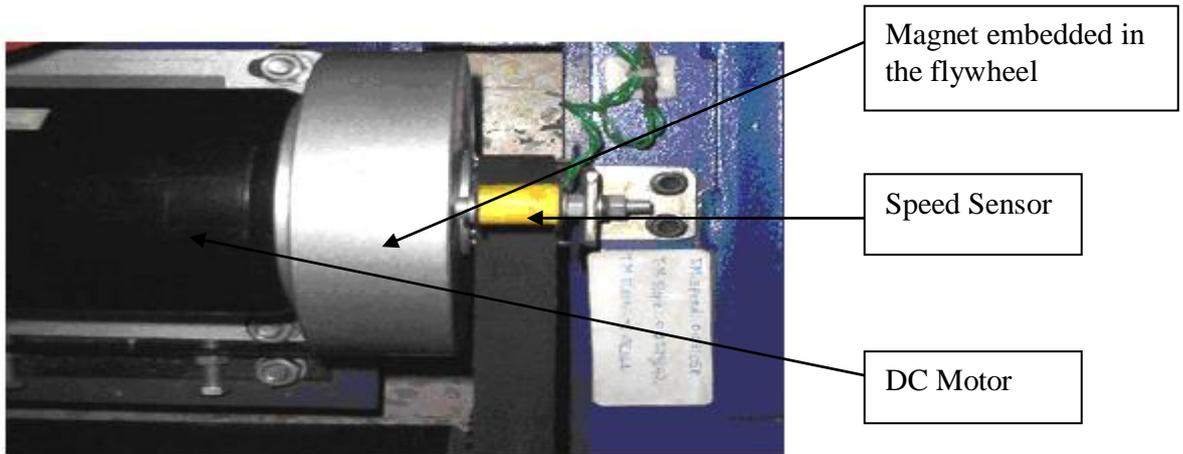
Fig 4. SPEED SENSOR
