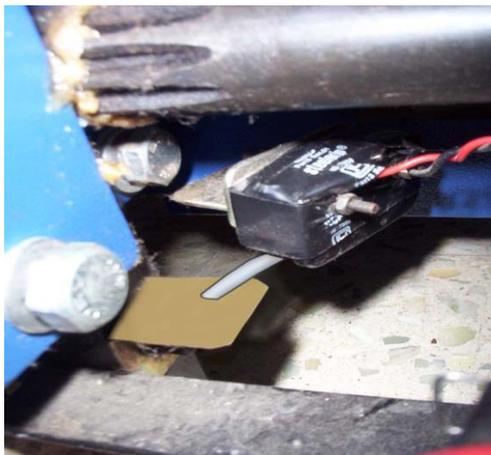
**Fig 8A. Limit switch clip at its original position.**
