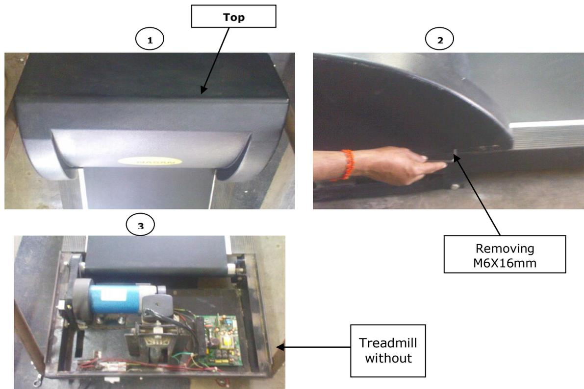
Fig.12.Treadmill after removing top cover
