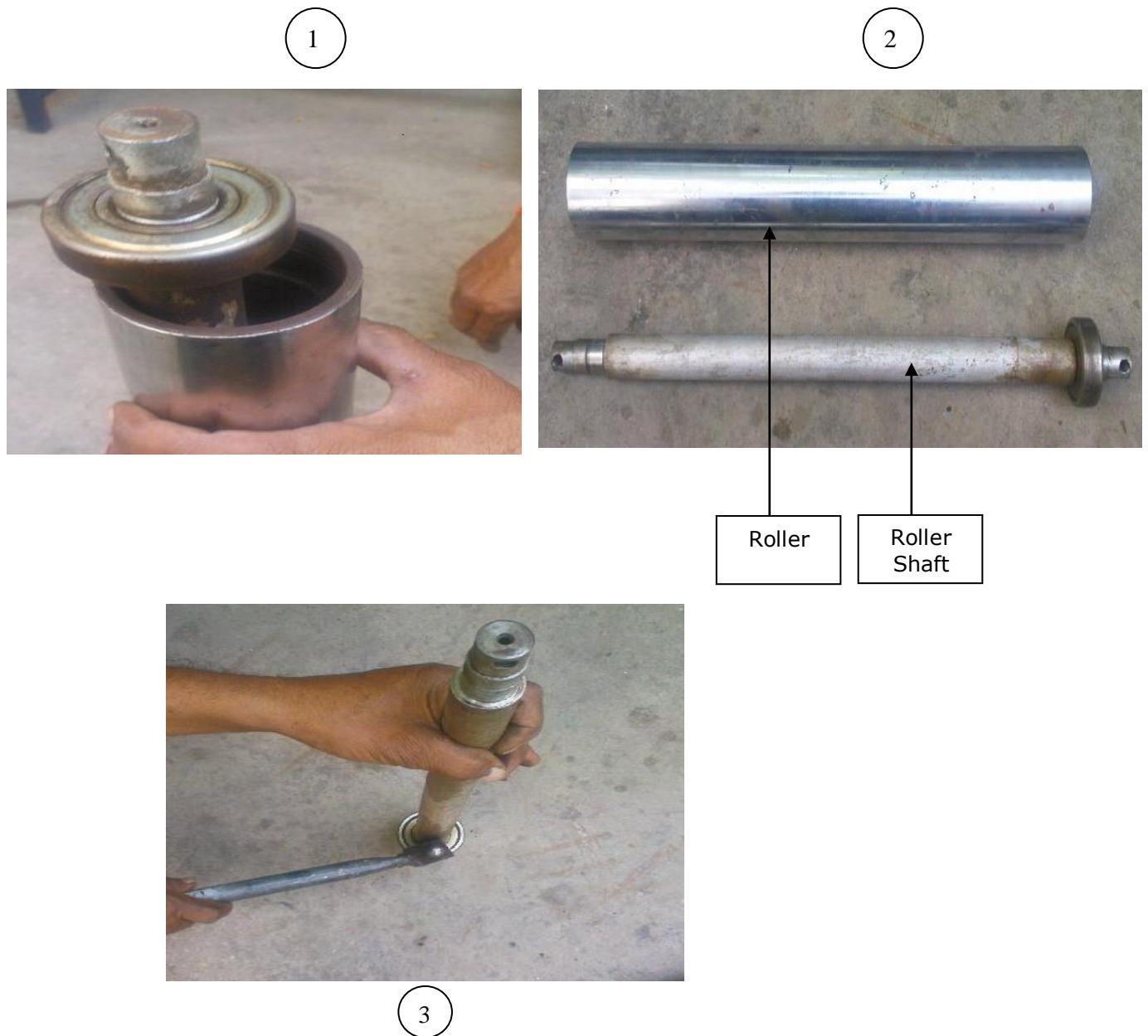
**Fig.20: - Removing Bearing from Roller.**
