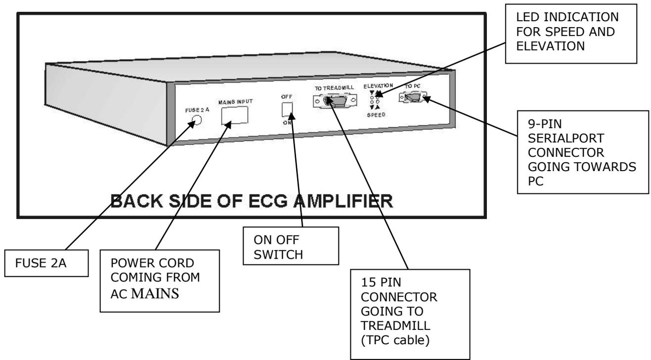
**Fig 2. AMPLIFIER CONNECTIONS**
