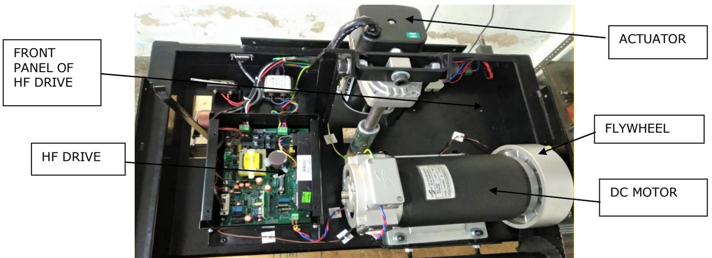
**Fig 4. TOP VIEW OF HIGH FREQUENCY (HF) DRIVE**
