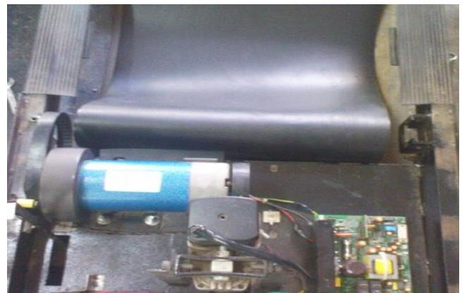
**Fig.18. Treadmill after removing front roller**
