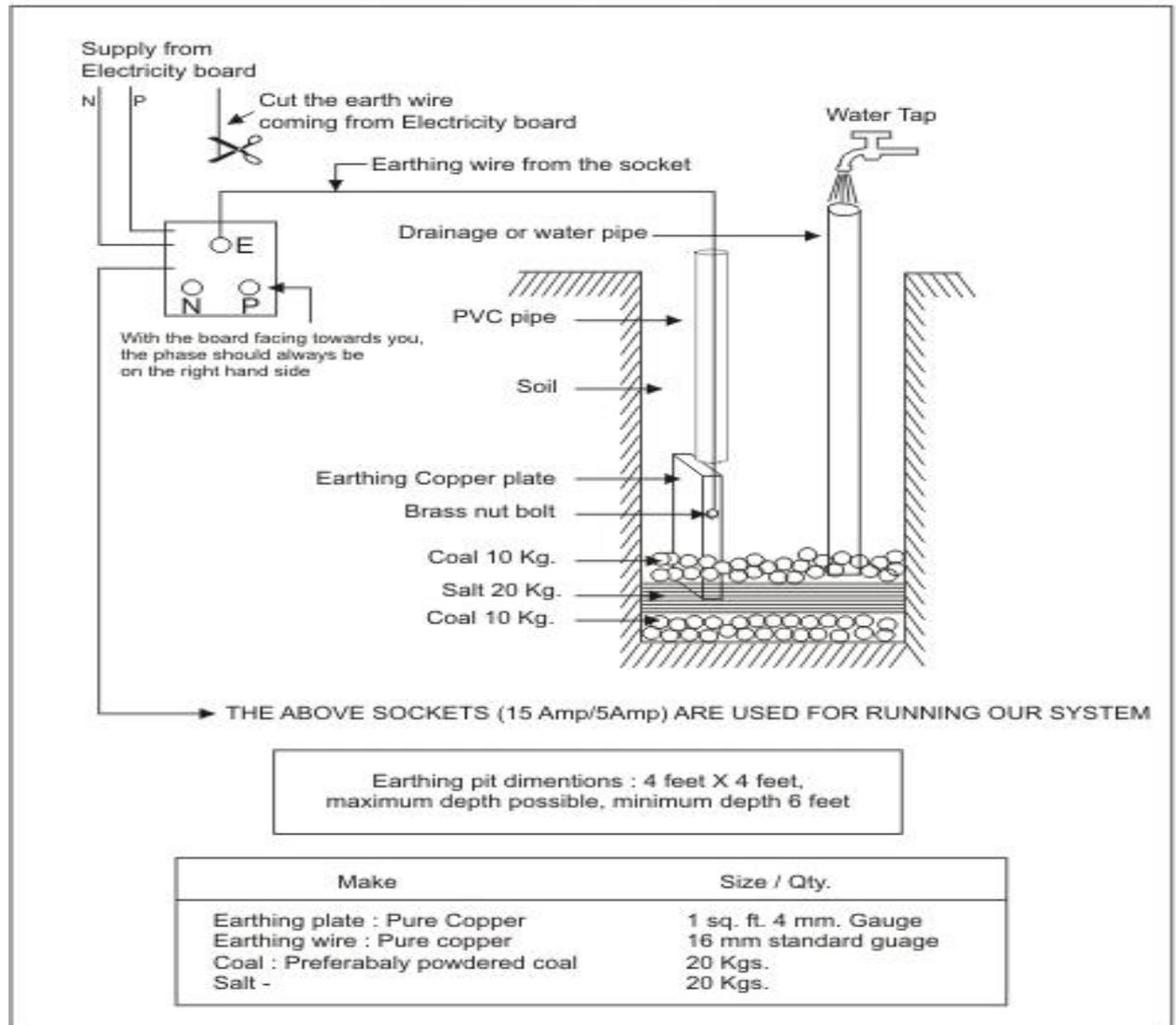
Earthing should be preferably done near the drainage system else there should be frequent watering of earth pit once in 5 months
