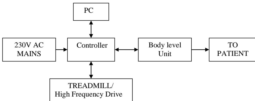
**Fig 1. BLOCK DIG. OF Treadmill Controller SYSTEM**
