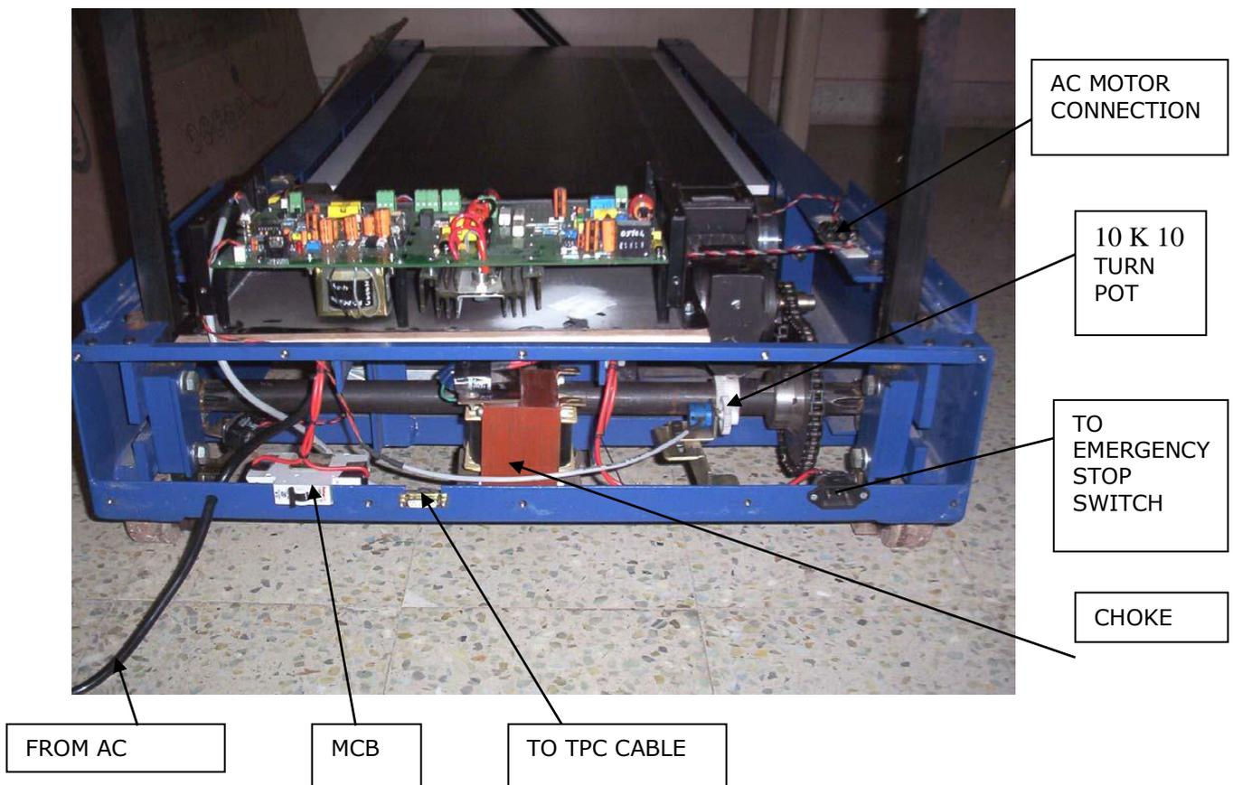
**Fig 6. FRONT PANEL CONNECTION**
