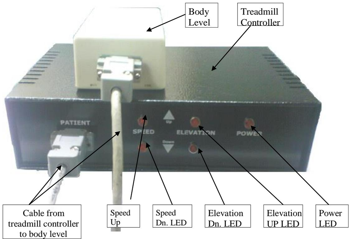
**Fig 2. Treadmill Controller + Body level system.**
