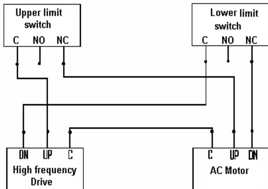
**Fig 8. Limit switch connections for compact machine.**
