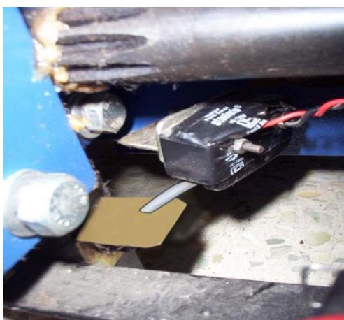
**Fig 8A. Limit switch clip at its original position.**
