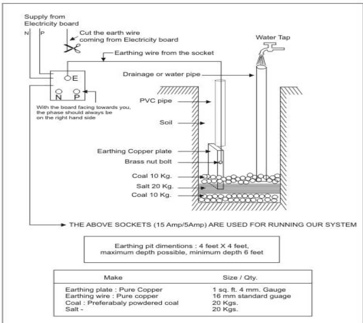
Earthing should be preferably done near the drainage system else there should be frequent watering of earth pit once in 5 months
