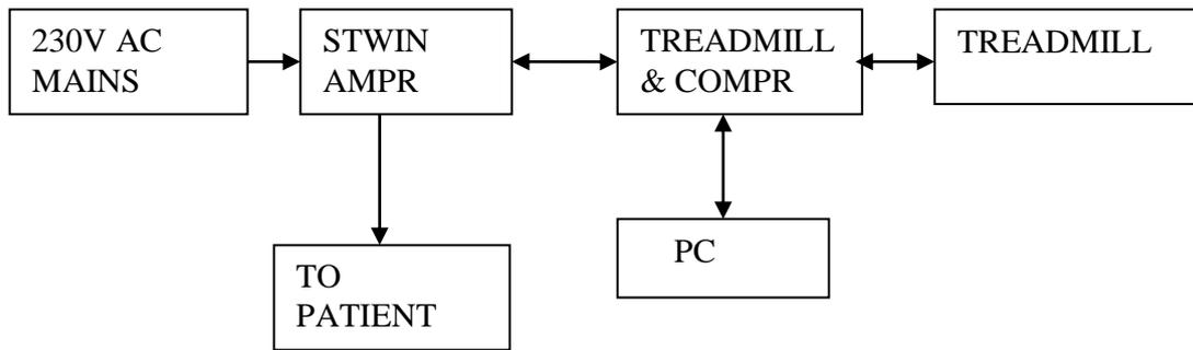
**Fig 1. BLOCK DIAGRAM OF ST-WIN SYSTEM**
