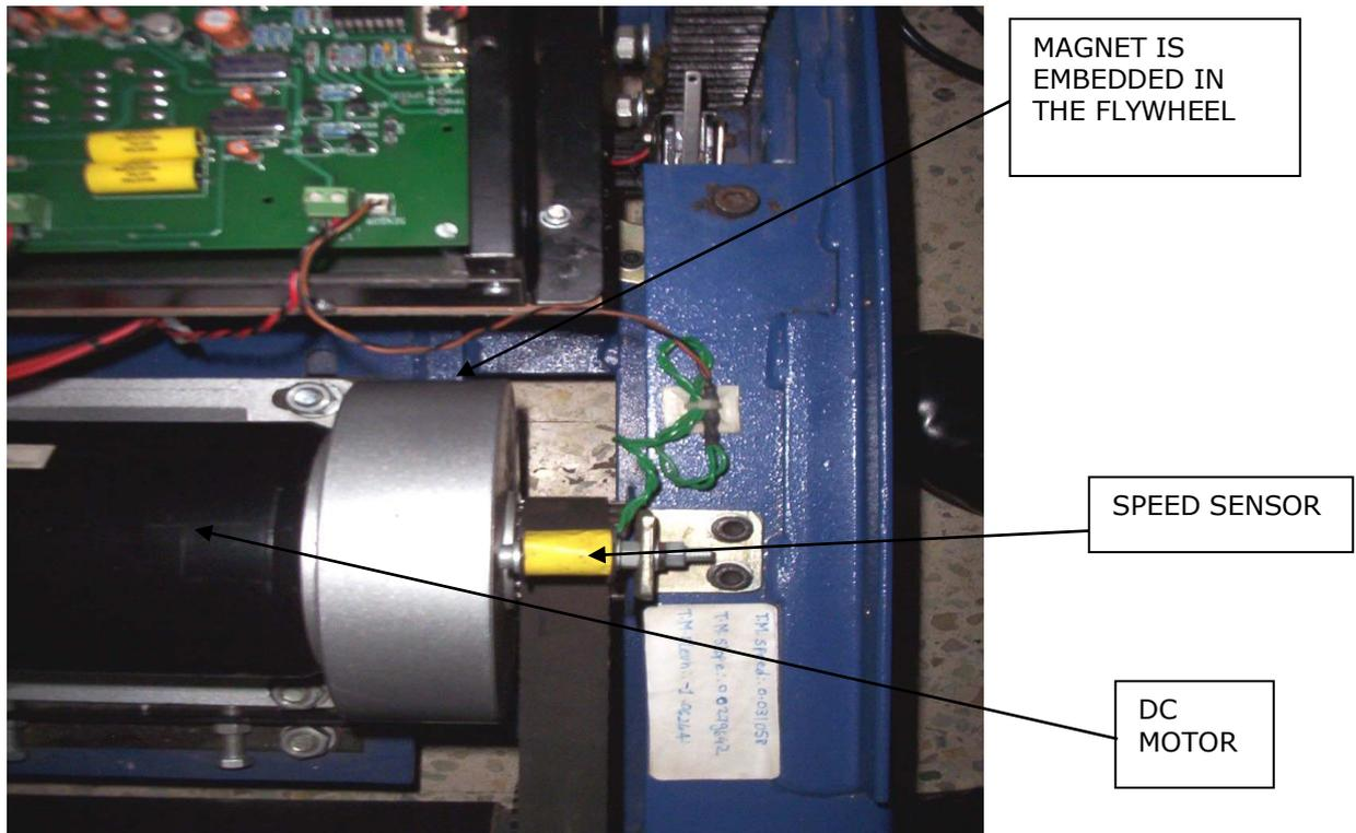
**Fig 5. SPEED SENSOR**
