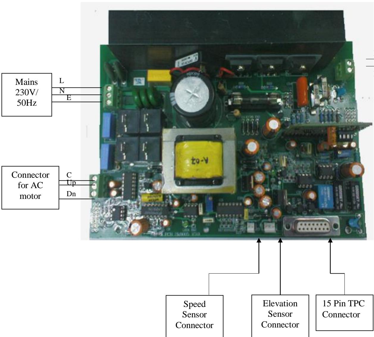
**Fig 7. High frequency drive connections**
