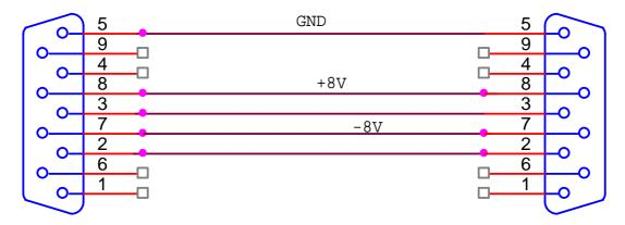
9 pin D Type Male connector on the BLA box 9 pin D Type Male connector on the TMC box
